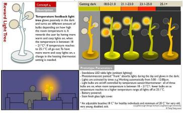
Colour changing Light indicates the room temperature (<27° C: brighter cold; 18 – 21° C: bright warm; 22 – 24° c: dim cold; 25° C<: off)
